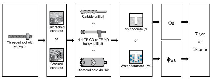
FIGURE 3—FLOWCHART FOR THE ESTABLISHMENT OF DESIGN BOND STRENGTH
